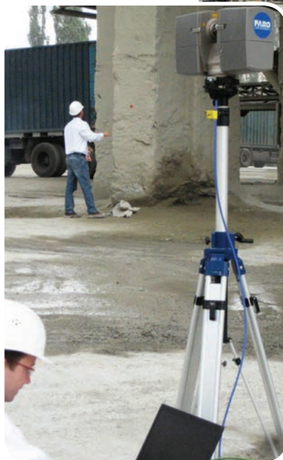
Above: in only one single visit to the site, plant components and existing buildings can be measured with an accuracy of within millimetres and recorded as digital data, which can subsequently be assembled in a cluster representation
