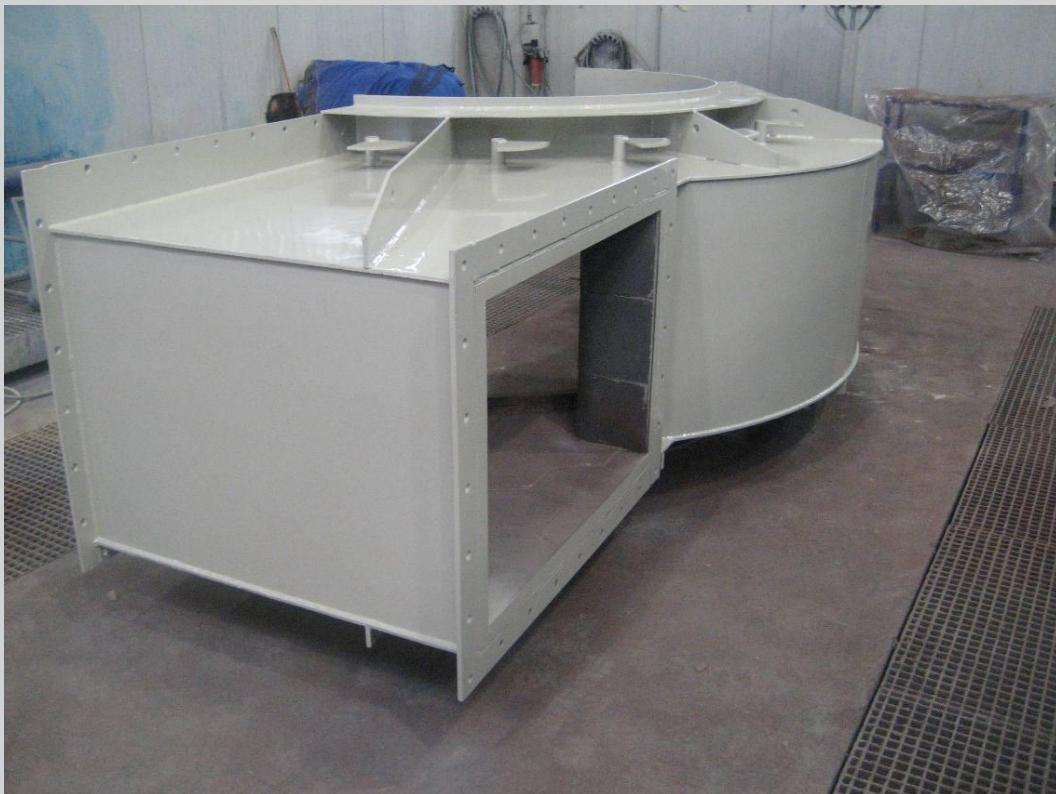
Seperator casing (after refurbishing)
