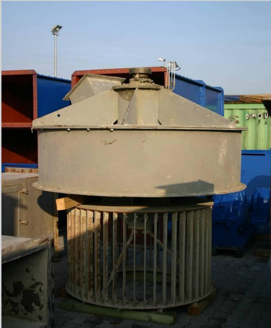
Cage wheel of the separator (after dismantling)
