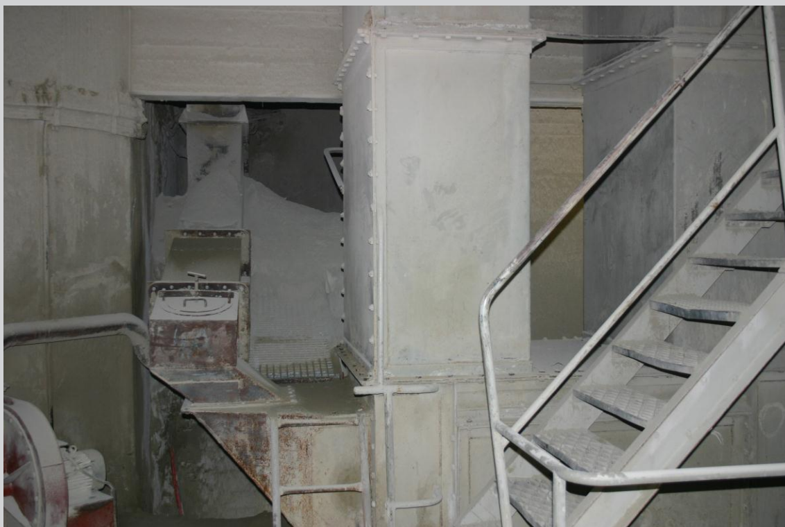
Bucket elevator with feeding air slide (Original place of installation)
